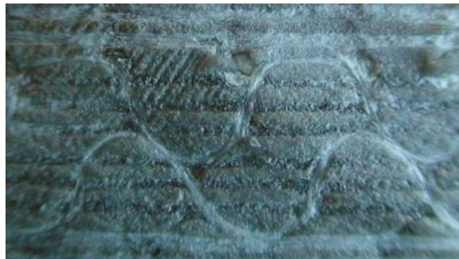
Fig. 3 Nesting of two adjacent layers of 3250 \text{ g/m}^2 (7 layer 90^\circ/0^\circ/90^\circ/0^\circ/90^\circ/0^\circ/90^\circ ) 3D woven reinforcement.
